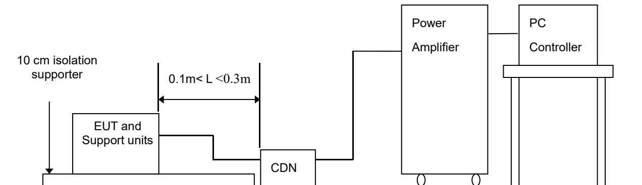
**Note:** 1. The EUT is setup 0.1m above Ground Reference Plane
